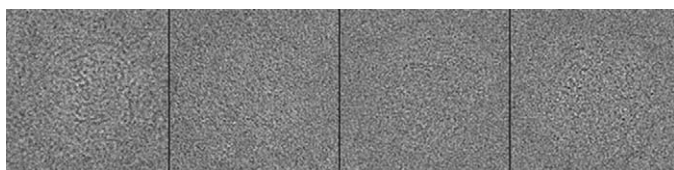
Fig. 4. Representative RDV raw images (from close-to-focus micrographs) collected in a JEOL 4000 electron microscope. Image size is 300 \times 300 pixels with 2.8 Å/pixel.
